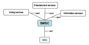
The Teligent SMSC offers an extensive range of interfaces that can be used for interconnection with other systems and 3rd party services. There is also multiple network support for GSM and TDMS/CDMA
