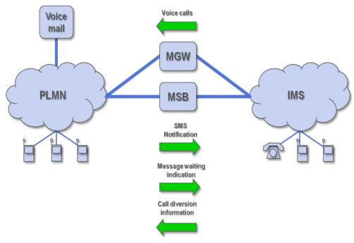
In addition to mobile/fixed and IMS/SIP service interaction the MSB is also capable of providing service interaction between fixed and mobile networks. The possibilities for further service offerings based on existing platforms, as well as cross network pre-paid billing interaction, open up a whole new range of possibilities for the operator to build and expand on existing investments.
